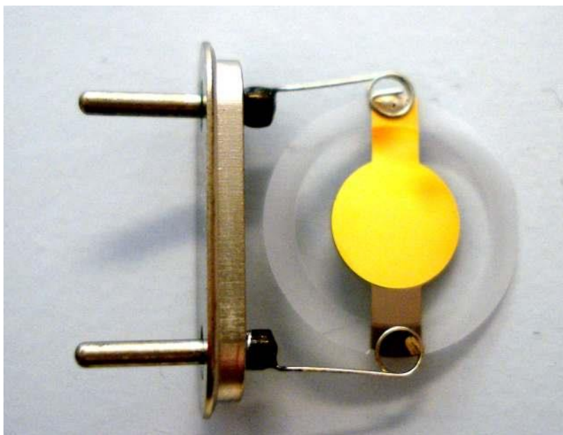
Figure 3 – Schematic view of the quartz crystals
